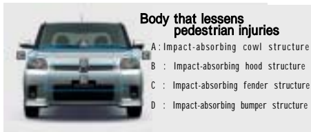
Body of new Corolla Rumian lessens pedestrian injuries
