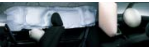
Airbags in the new Corolla Rumian
